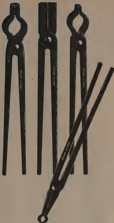
Heller blacksmith's tongs from the makers of the first U.S. anvil, Fisher and Norris.
